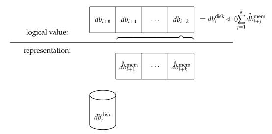
As depicted above, the representation consists of a single disk state and a series of in-memory differences. Each difference is the individual difference from performing a transaction. That is, we keep each difference and do not compose them together prematurely. Each logical database
