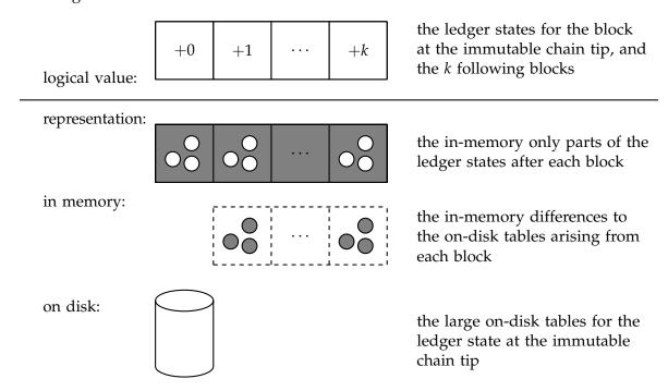
This design resolves the tension: it uses only a single on-disk value at any one time, which lets us use traditional database techniques, and yet it also lets us efficiently work with multiple logical values of the database state at once.
