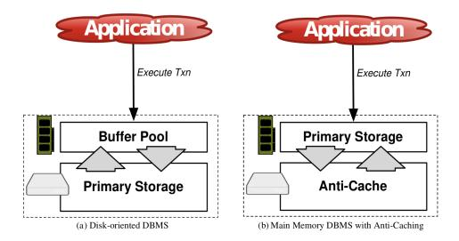
Diagram by DeBrabant et al. [2013, Figure 1] illustrating the difference in database architecture: "In (a), the disk is the primary storage for the database and data is brought into main memory as it is needed. With the anti-caching model in (b), memory is the primary storage and cold data is evicted to disk."
