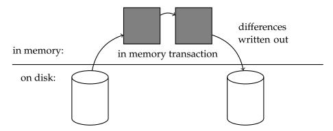
The simplest scheme, as in the diagram above, would be to write differences back to disk immediately. As we will discuss, we will actually want to hold the differences in memory across many transactions and flush them to disk later.
